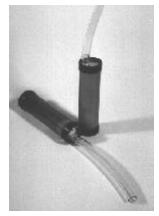
The simplest to use is the Breath Builder. Developed by Bassoonist Harold Hansen of Las Vegas, Nevada, the Breath Builder is a device used to feel the sensation of inhaling and exhaling. It is a tube of plastic [at least six inches tall] with a ping-pong ball inside. The bottom is sealed and the top has three holes drilled to vary the resistance.
